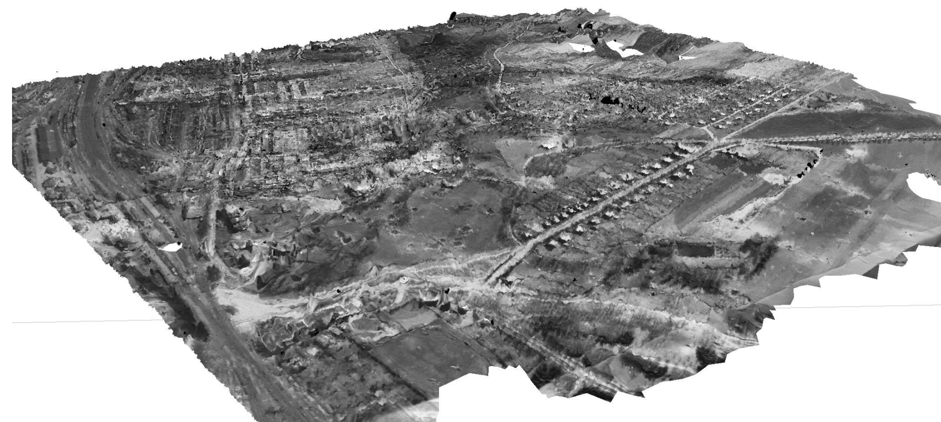
Fig. 2: Created Model from the Gotha case study based on DL Feature Matching
