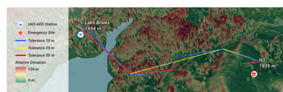
Flight plan simulation using different simplification parameters over steep slopes
