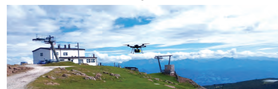
Flight test to deliver a defibrillator using paths adapted to the terrain (July, 2023)
