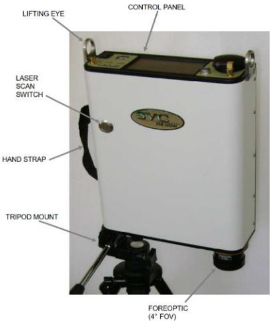
Fig. 16 (A) SVC HR-1024i and (B) LC-RP PRO
