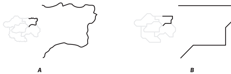
Figure 2.12.: Increased angular legibility by schematization: the magnified polygon boundary of the schematized region B expose fewer, but longer edges than the generalized region A . Furthermore, angles close to 0^\circ or 180^\circ do not occur.
