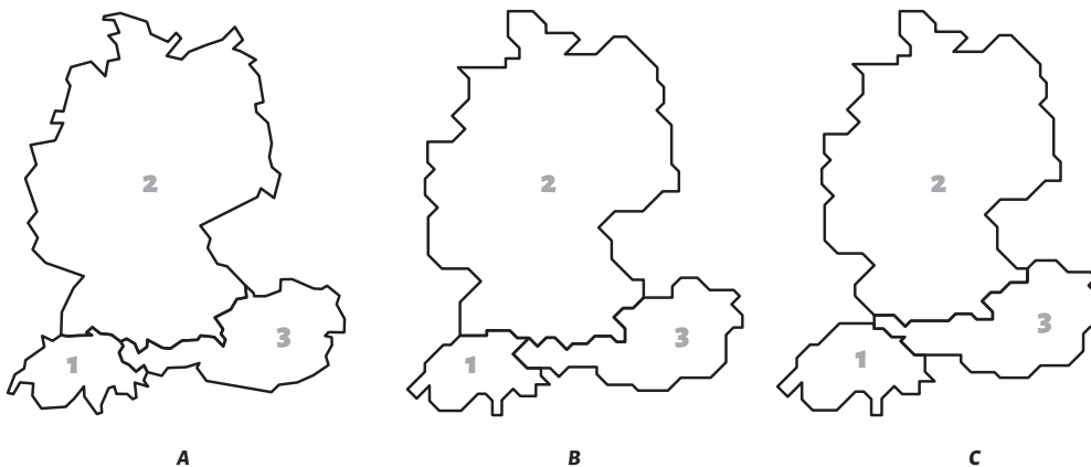
Figure 2.7.: A In the original input polygon 1 and 2, 1 and 3, and polygon 2 and 3 share one border each. The same adjacencies are present in B , making it a topology preserving schematization of A . C shows a schematization where polygon 1 and 2 do not have any edge in common, thus a schematization which does not preserve topology.
