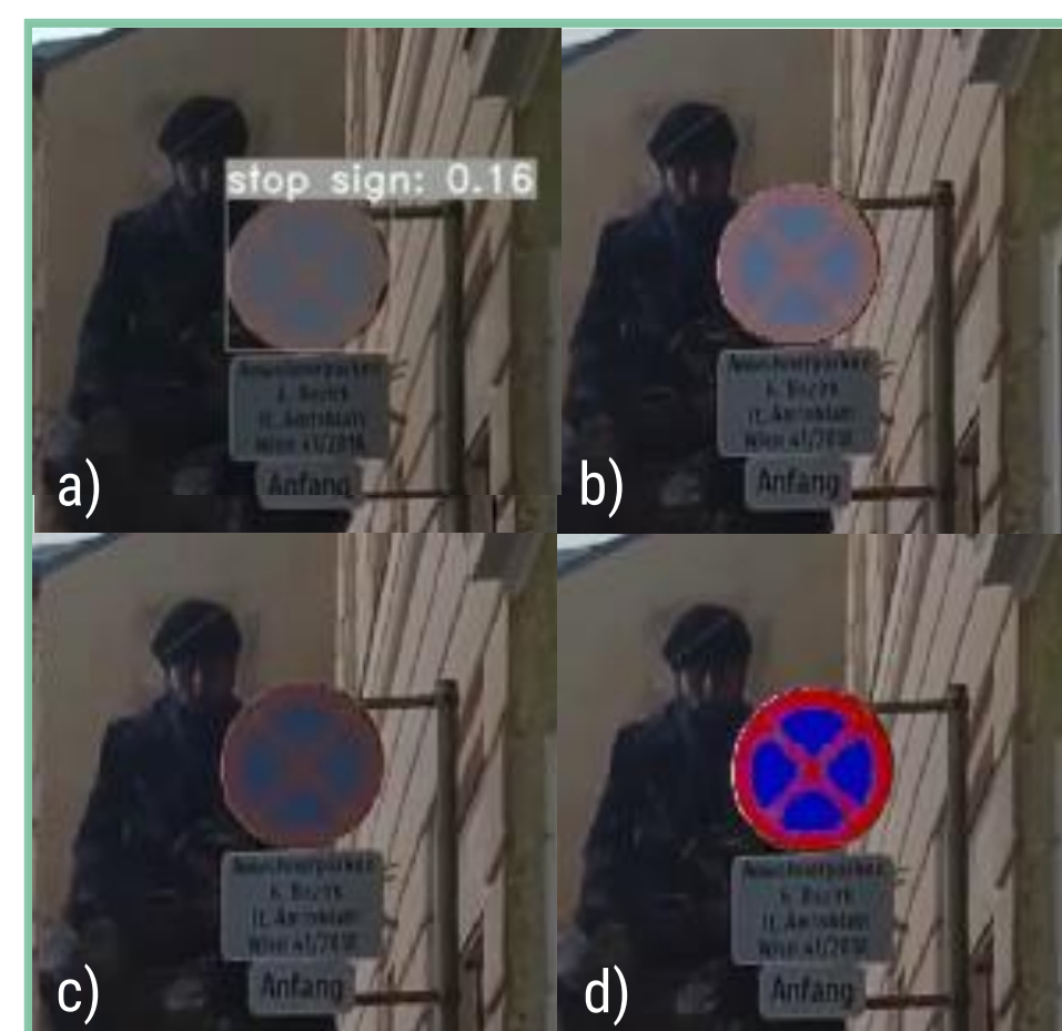
Figure 2. Techniques to highlight object features: a) detected object b) brightness enhancement c) contrast enhancement d) saturation enhancement.
