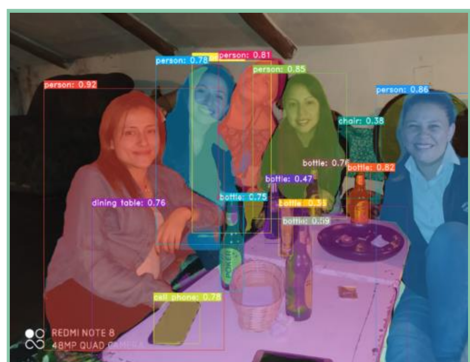
Figure 1. Instance segmentation of objects in imagery employing YOLACT (You Only Look At Coefficient).
