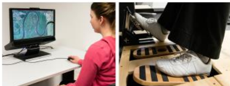
Figure 11: Gaze-supported Foot Navigation, using foot-rockers and foot-pedals (Klamka et al. 2015)
