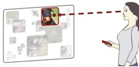
Figure 1. Basic idea: Gaze-supported interaction in combination with a handheld touchscreen and a distant display.
