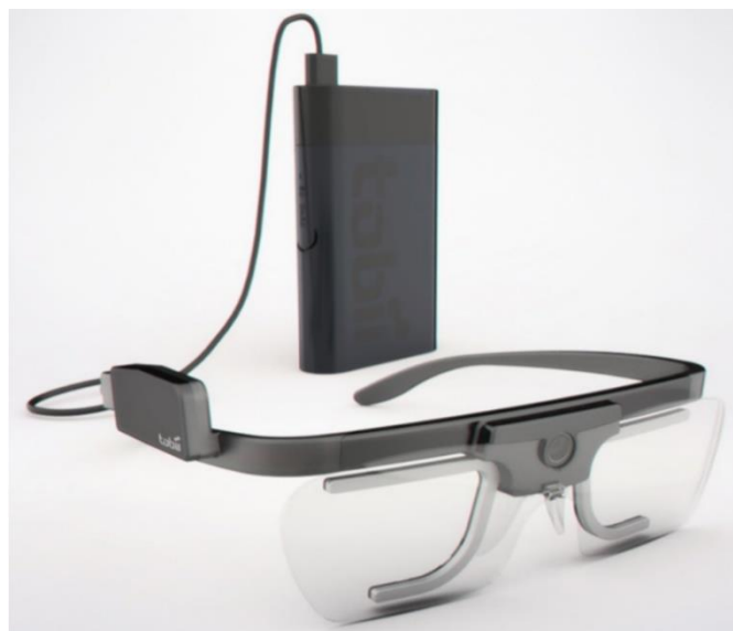
Figure 5.1 Tobii 2 Pro Eye-Tracking Glasses: recoding unit and head unit (Source: URL15)
