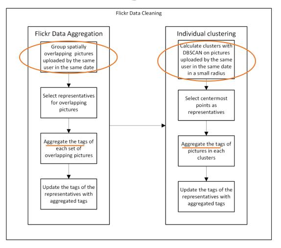
After experiments, parameters for DBSCAN: Epsilon = 30 meters
