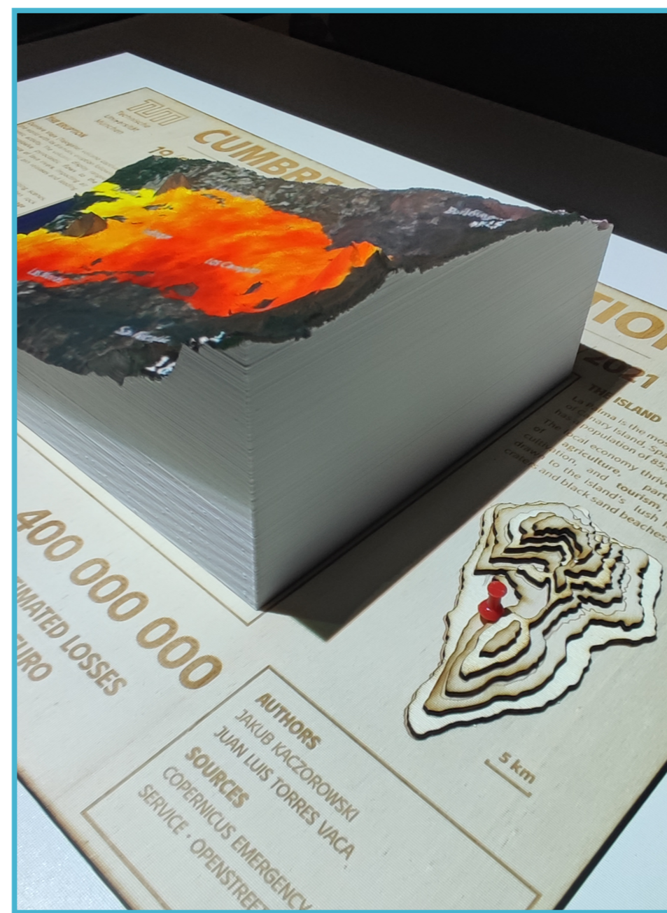
Fig 2. Photo of the final product: laser-engraved base, 3D print with projection and laser-cut contour map
