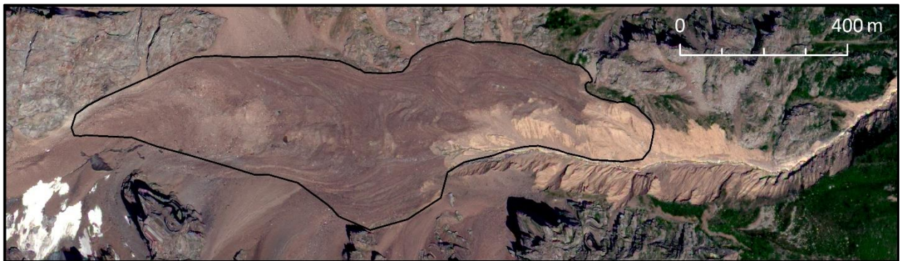
Figure 52: A rock glacier with a large debris flow scar. The lower part of the rock glacier was washed away.
