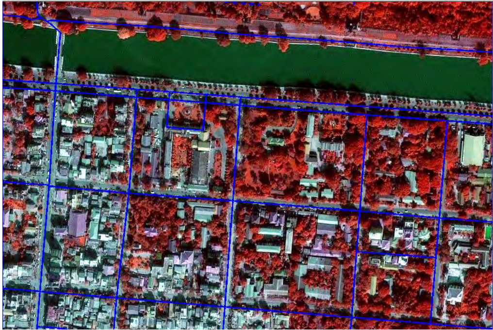
Figure 10: Result of first segmentation – Chessboard Segmentation using OSM road network on ROAD_SEGMENT level
