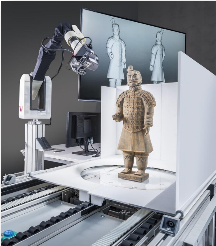
Figure 04: Photogrammetric system (Fraunhofer IGD - CHD, 2017)
