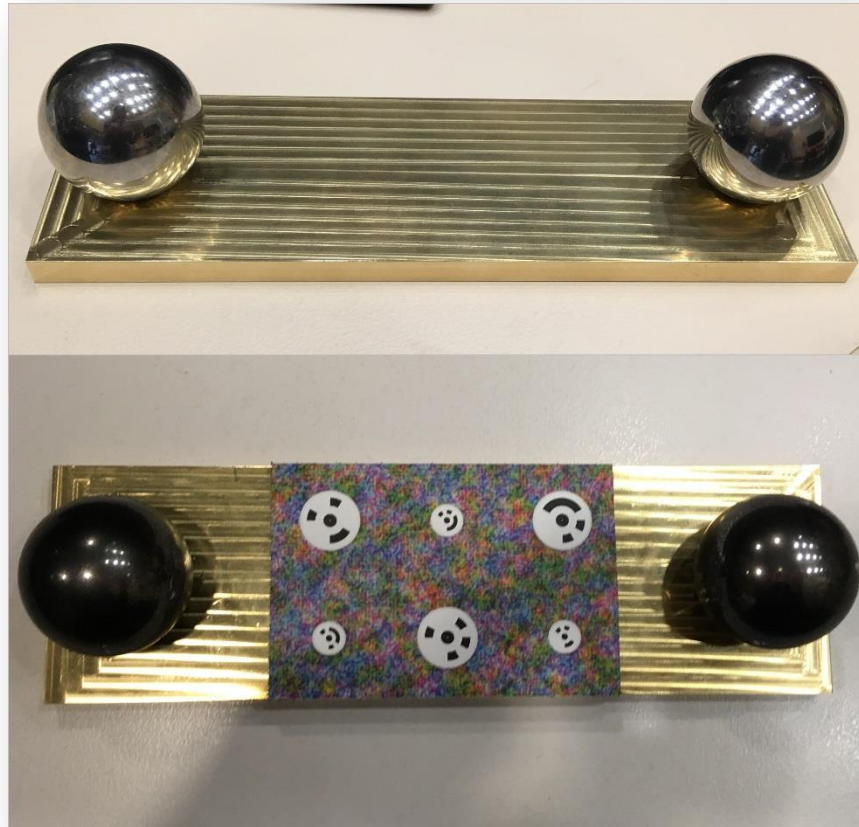
Figure 07: Sphere plate before and after its preparation
