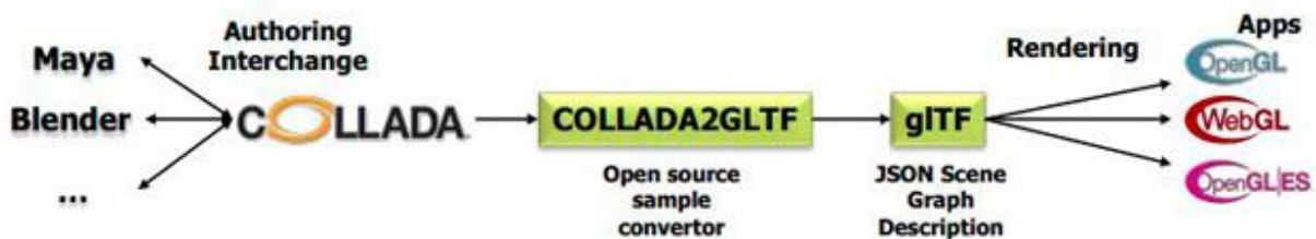
Figure 2-7: glTF pipeline progression of content authoring, conversion, delivery, rendering (Trevett, 2013)
