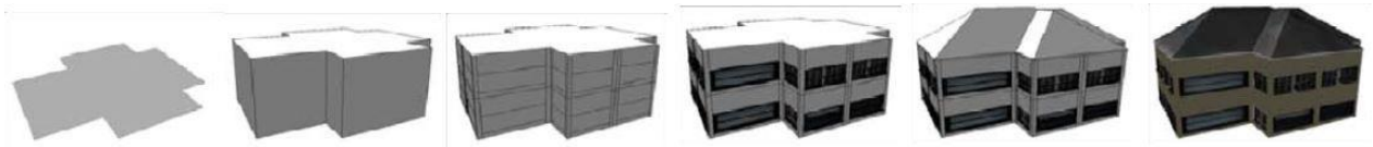
Figure 2-5: Principle of the procedural modeling (Radies 2013a)
