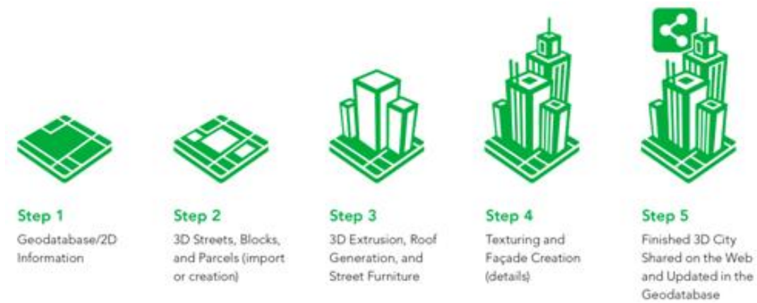
Figure 2-15: Creation steps of a 3D city model in the CityEngine software (Esri n.d.(b))
