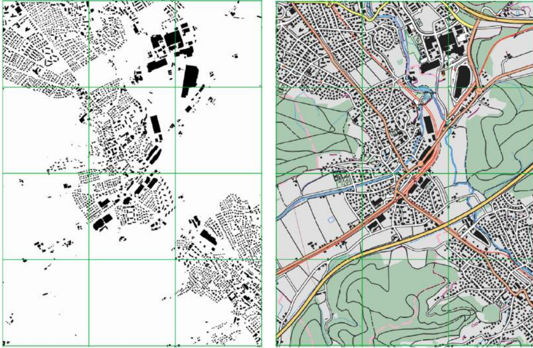
Figure 4.13: Left side: TLM data; Right side: 1:50'000 map extract, buildings obtained fully automatically
