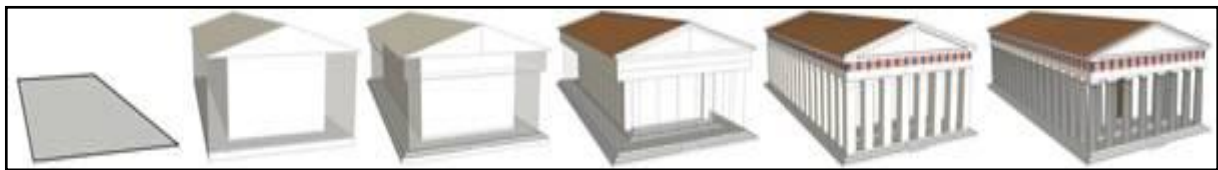
Figure 16: shows the rule derivation which start from the left with the start shape and on the right with the result of the generated model.
