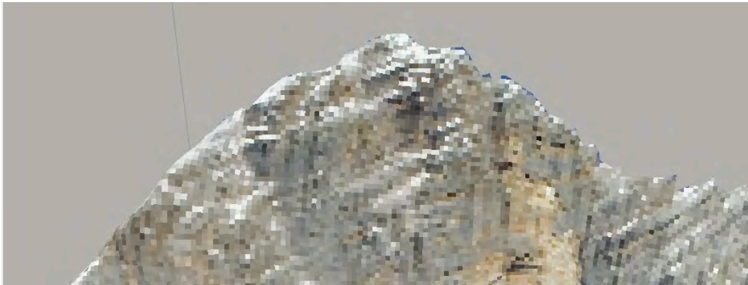
Figure 5.19 Low-resolution texture due to Texture Atlas settings
