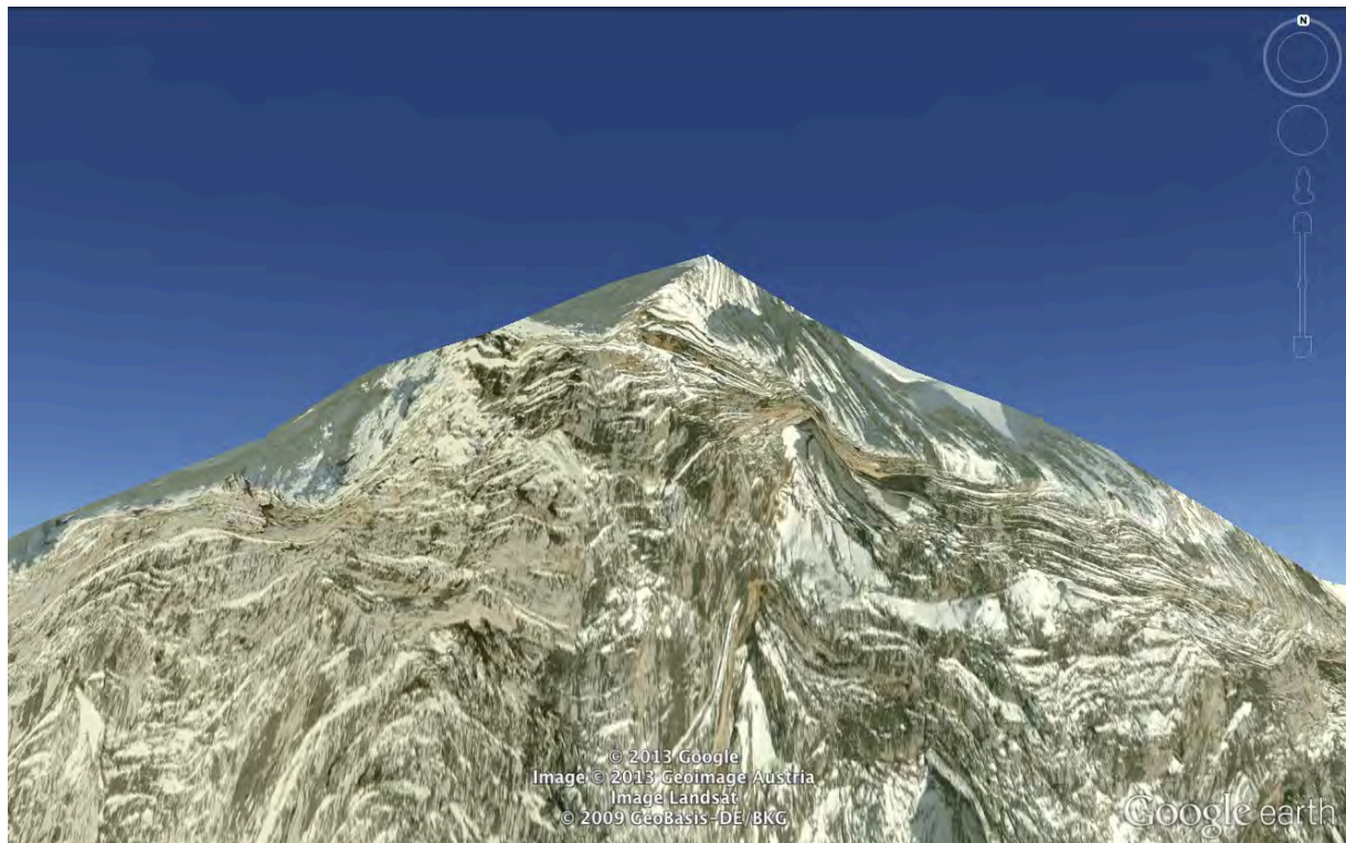
Figure 2.2 Low density TIN – Inset view of Hoher Dachstein showing distortion of texture
