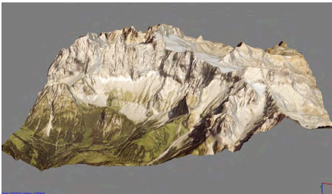
Figure 4.5 Dachstein Massif reconstructed with SfM using nadir photos
