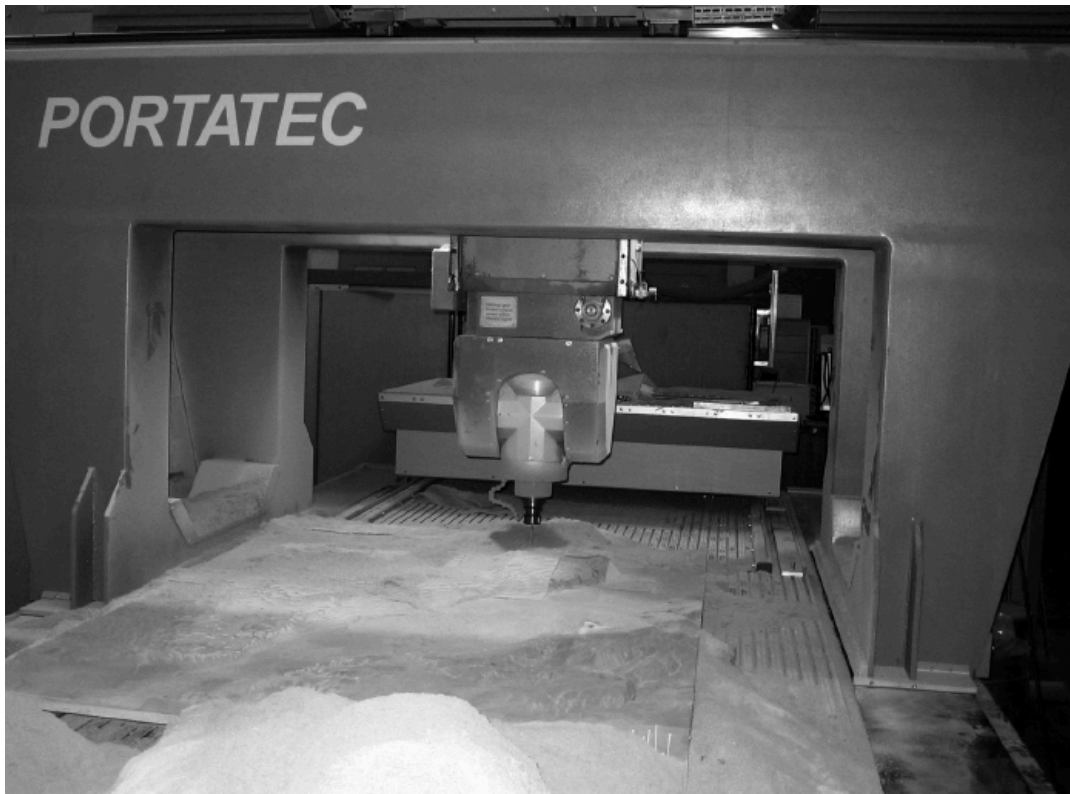
Figure 4.8 Creating an STM with a CNC milling machine
