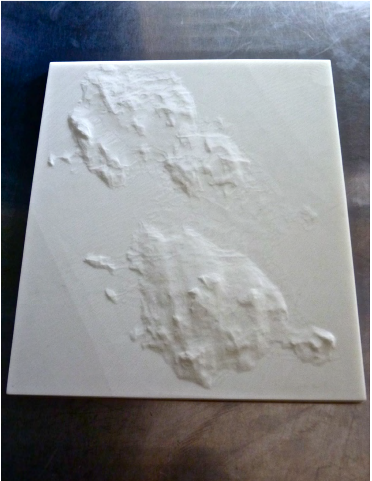
A3.4 Topographic relief model after the CNC milling process
