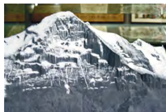
Figure 3: Lack of detail on vertical surfaces when 3D printed model is created from DEM data. (Photo: T. Mair)
